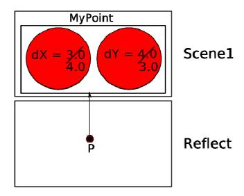
The parameter P is a reference to the object named MyPoint. The usual representation for a reference is a dot with an arrow that points to whatever the reference refers to.
